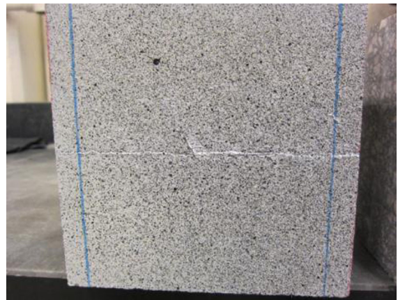
Fig. 8 Speckled surface of a shear specimen
