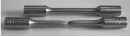
Figure 5.23 Tensile testing specimens.
